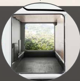
Tall rear garage with access from both sides and max. 150 kg distributed load
