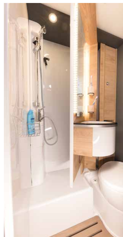
To transform the bathroom into a shower cubicle, simply release the lock and swing the swivel wall out over the toilet.
