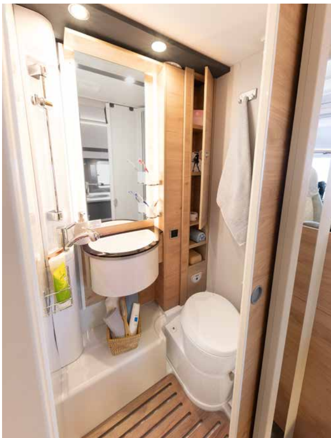
The bathroom in the basic position! The swivel wall nestles against the outer wall to save space and thus ensures plenty of elbow room.
