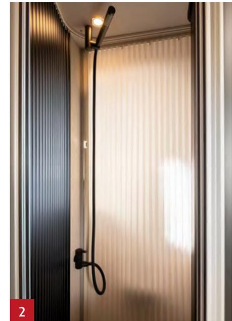
**1 Swivel bathroom:** the spacious bathroom with swivel wall offers extra freedom of movement when showering. The specially shaped swivel wall maximises the available space when showering without taking up space in the bathroom when the sink is in the useable position.
