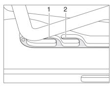
Fig. 35 Heki skylight in ventilation position
