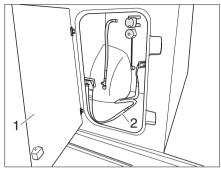
Fig. 59 Access flap for the gas bottle
