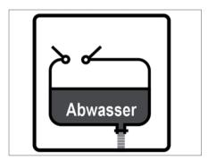
Fig. 100 Waste water tank symbol
