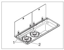
Fig. 85 Operating controls for gas cooker
