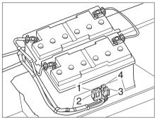
Fig. 75 Fuses in the battery box
