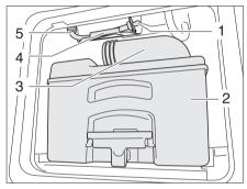
Fig. 111 Toilet water tank drain hose
