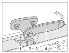
Fig. 19 Catch lever with safety knob in "closed" position
