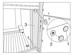
Fig. 113 Cover in the vehicle rear
