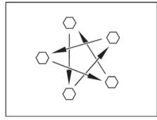
Fig. 115 Tighten the wheel nuts or wheel bolts cross-wise
