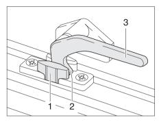
Fig. 21 Catch lever in the "continuous ventilation" position
