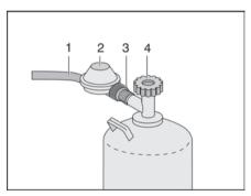
Fig. 60 Gas bottle connection
