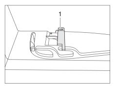
Fig. 36 Ventilation position locking mechanism
