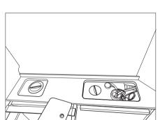
Fig. 95 Water tank (CVD540/600)
