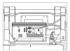
Fig. 73 Fuse under the driver's seat
