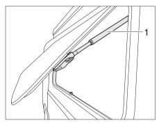
Fig. 29 Hinged window with damping, opened
