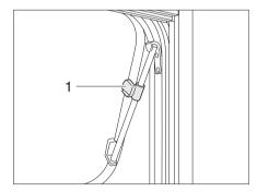
Fig. 20 Hinged window with rotary hinges, open
