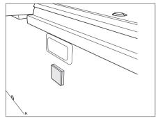
Fig. 49 12 V socket and light in the rear on the left side (CVD540)
