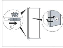
Fig. 93 Dometic locking mechanism of the refrigerator door
