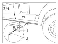
Fig. 99 Operation of the waste water tap
