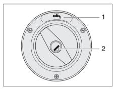
Fig. 15 Cap for the fresh water filler neck (Variant 1)
