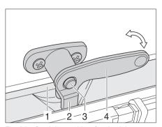
Fig. 24 Catch lever with safety knob in "closed" position
