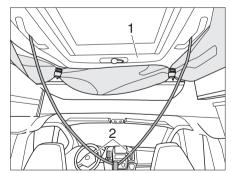
Fig. 58 Closing the pop-up roof
