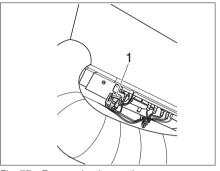
Fig. 77 Fuse under the seating group
