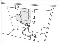
Fig. 78 230 V automatic circuit breaker
