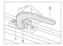
Fig. 23 Catch lever in "closed" position
