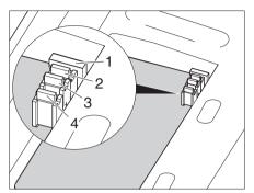
Fig. 74 Fuses on the starter battery
