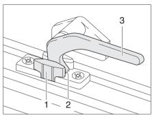
Fig. 26 Catch lever in the "continuous ventilation" position
