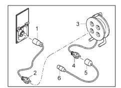
Fig. 71 Connection options for 230 V power connection
