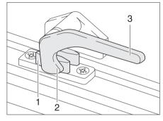
Fig. 18 Catch lever in "closed" position
