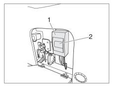
Fig. 79 230 V automatic circuit breaker (CVD540/600)
