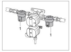
Fig. 68 High-pressure hoses with hose break guard (country-specific variants)
