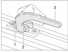
Fig. 28 Catch lever in "closed" position
