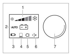
Fig. 88 Operating controls for the refrigerator (Dometic 10 series)
