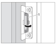
Fig. 92 Turning the locking mechanism back to the initial position
