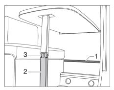
Fig. 40 Suspension table with fold-out leg
