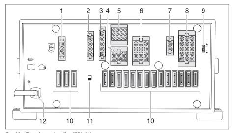
Fig. 69 Transformer/rectifier (EBL 31)
