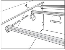
Fig. 52 Slatted frame support bars
