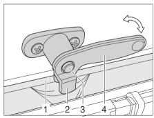
Fig. 27 Catch lever with safety knob in "Continuous ventilation" position
