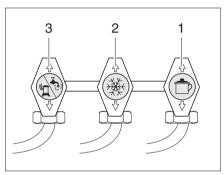
Fig. 80 Symbols for the gas isolator taps
