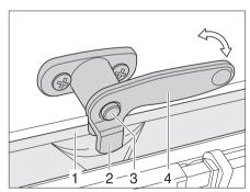
Fig. 22 Catch lever with safety knob in "Continuous ventilation" position
