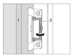
Fig. 91 Locking in the ventilation position
