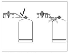
Fig. 64 Routing the high-pressure hoses
